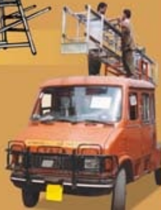
Aluminium Telescopic Tower Ladder Size 8' to 40' (HI 160)
